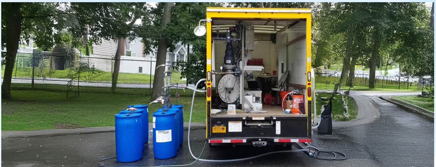
Figure 15: A mobile UV AOP system used for on-site pilot and performance testing.
