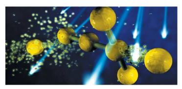
UV breaks down the bonds of chlorine & chloramine molecules to reduce their levels down to parts per billion.
