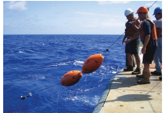
SBE 37 MicroCAT CTD on a mooring line, being deployed from a ship
