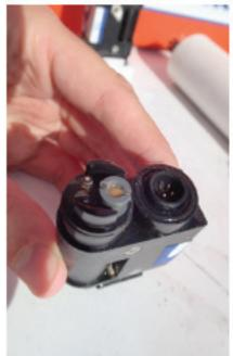
The pictures to the left show the outside of an instrument deployed at Shilshole Bay as well as what the pH sensor looks like when removed from the internal flow path. The internal pump and flow path used in the HydroCAT-EP help protect the pH sensor from accumulating biological growth, therefore limiting drift due to biofouling.
