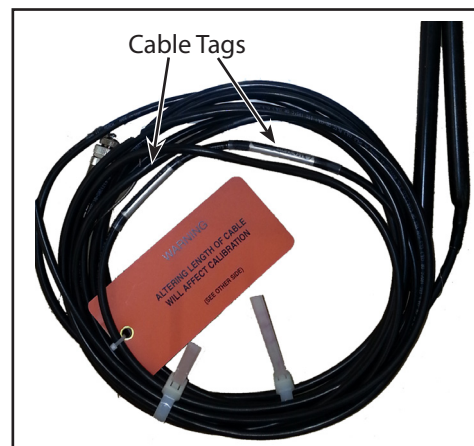
Figure 4. Cables with Cable Tags
