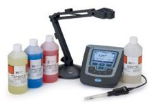
Portable and laboratory **HQD Meters** determine pH, conductivity, dissolved oxygen and ORP. They are connected to smart interchangeable Intellical probes for quick, simple, and reliable measurements.
