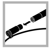
**4.** Put the probe in the calibration and storage chamber. Make sure that the probe tip stays dry.
