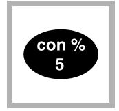
7. To change the units that show on the display (mg/L or % saturation), push con %.
