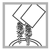
**9.** Add two 10-mL DPD Free Chlorine Reagent Powder Pillows or two 10-mL DPD Total Chlorine Reagent Powder Pillows to the second sample cell.
