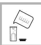
2. Prepare the blank: Rinse a 1-cm/10-mL sample cell and cap three times with sample. Fill the sample cell to the 5-mL mark with sample. Close the sample cell.
