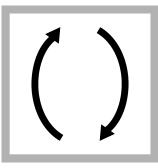
**10.** Close the sample cell. Invert the sample cell for about **20 seconds** to dissolve the reagent. Undissolved power will not affect accuracy.
