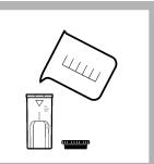
**8. Prepare the sample:** Rinse a second 1-cm/10-mL sample cell and cap three times with sample. Fill the sample cell to the 5-mL mark with sample.
