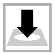
**14. Total chlorine measurement:** After 3 minutes and within 6 minutes of the reagent addition, insert the prepared sample into the cell holder. Point the triangle mark on the sample cell away from the keypad.
