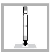
7. Insert the vial into the cell holder.DR1900: Go to LCK/TNTplus methods.Select the test, push READ.
