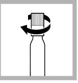
**4. Immediately** screw the DosiCap Zip back on; **fluting at the top**.
