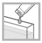
**8.** Pour the blank into the sample cell.
