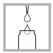
**4. Prepare the sample:** Use a pipet to add 3.5 mL of sample into the other test vial.
