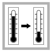
**9.** When the timer expires, carefully remove the vials from the reactor. Set the vials in a test tube rack. Let the temperature of the vials decrease to room temperature.
