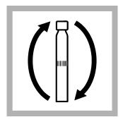
**12.** Tighten the cap on the vials and invert the vials 2–3 times.
