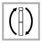
**5.** Tighten the cap on the vials and invert the vials 2–3 times.
