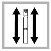
**6.** Shake each vial 2–3 times to dissolve the reagent in the cap. Look through the open end of the DosiCap to make sure that the reagent has dissolved.
