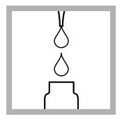
**3.** Use a pipet to add 0.2 mL of Solution B to each vial. Immediately tighten the cap on the Solution B container.
