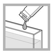
**15.** Pour the digested blank into the sample cell.
