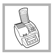
**7.** Insert the vials in the preheated DRB200 reactor. Close the lid.
