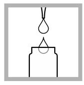
**2. Prepare the sample:** Use a pipet to add 3.5 mL of sample into the other test vial.
