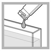
**20.** Pour the digested sample into a second sample cell.
