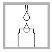
1. Prepare the blank: Use a pipet to add 3.5 mL of deionized water into one test vial.
