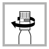
**5.** Turn the DosiCap Zip over the test vial so that the reagent side goes on the vial. Do this for each test vial, then tighten the caps on the vials.
