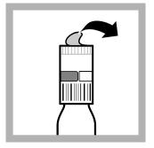
2. Carefully remove the lids from the DosiCap™ Zip caps. Remove the caps from the test vials.
