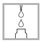
**10.** Use a pipet to add 0.2 mL of Solution B to each vial. Immediately tighten the cap on the Solution B container.
