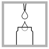
3. Prepare the blank: Use a pipet to add 3.5 mL of deionized water into one test vial
