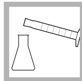
**4. Use a 100-mL graduated cylinder to measure 75 mL of concentrated sulfuric acid. Add the acid to a 250 mL plastic Erlenmeyer flask.**
