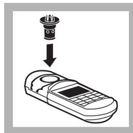
**3. Put the COD/TNT vial adapter in the cell holder. Rotate the adapter until it goes in. Then push the adapter down until click is heard.**
