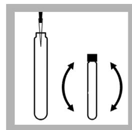
**8. Add 3.5 mL of the BoroVer 3 solution prepared in step 5 to the sample vial. Tighten the cap and immediately invert to mix.**
