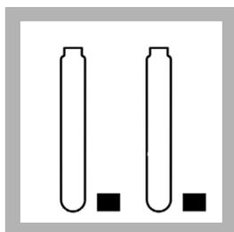
**6. Remove the caps from two clean 16-mm screw-capped vials. Refer to "How to use and clean glass vials" on page 2.**
