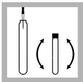
9. Add 3.5 mL of the BoroVer 3 solution prepared in step 5 to the blank vial. Tighten the cap and invert to mix.
