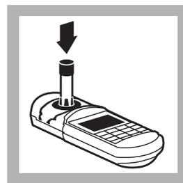
12. After the timer beeps, put the **blank** into the adapter. Push straight down on the top of the vial until it is fully installed. The vial must not move, because this can cause reading errors.
