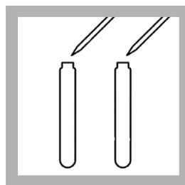
**7. Add 0.2 mL of sample to one vial (the sample) and 0.2 mL of deionized water to the other vial (the blank).**
