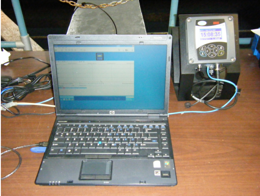
Figure 8. Data collection system including notebook PC and sc100 used for backwash study.
