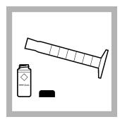
**5.** Fill a sample cell with 10 mL of the prepared sample.
