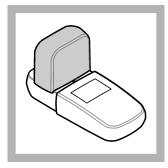
**12.** Install the instrument cap over the cell holder.
