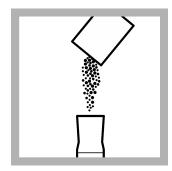
**3.** Add the contents of one Molybdenum 1 Reagent Powder Pillow to the mixing cylinder.
