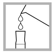
2. Prepare the sample: Fill a 25-mL graduated mixing cylinder with 20 mL of sample.
