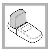
**17.** Install the instrument cap over the cell holder.
