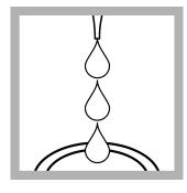
**6. Develop the sample:** Add 0.5 mL of Molybdenum 2 Reagent Solution to the prepared sample cell.
