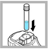
**12.** Put the sample vial in the vial adapter.
