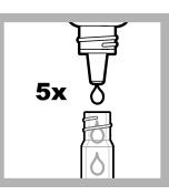
8. Add 5 drops of Fluorescence Free Chlorine **Reagent 2**. Hold the bottle vertically.
