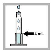
**9.** Put the sample vial in the sample vial holder. Add the sample to the top of the sample vial holder (4 mL).
