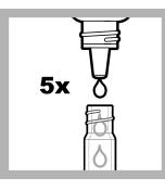
7. Add 5 drops of Fluorescence Free Chlorine **Reagent 1**. Hold the bottle vertically.
