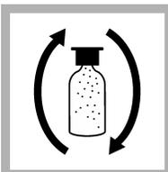
5. Put the cap on the tip of the ampule. Invert several times to mix. The blue color becomes lighter if ozone is in the sample.
