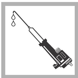
2. Hold the Digital Titrator vertically with the cartridge tip up. Turn the delivery knob to eject air and a few drops of titrant. Reset the counter to zero and clean the tip.
