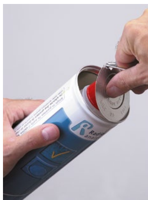
pH buffers can be stored in sealed cans for up to two years.
