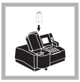
**15.** Place the blank into the cell holder. Close the light shield.
