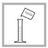
**3.** Measure 300 mL of deionized water in a 500-mL graduated cylinder.
