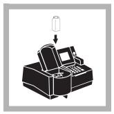
17. Place the prepared sample into the cell holder. Close the light shield. Result in mg/L phenols (or chosen units) will be displayed.
