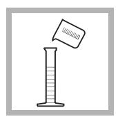
**5.** Measure 300 mL of sample in a 500-mL graduated cylinder.
