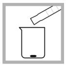
3. Without excessive agitation, measure 200 mL of sample with a clean graduated cylinder.
