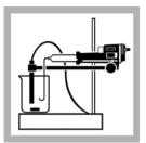
10. Continue the titration, recording at least three points on the downward sloping curve and at least three points after the end point is reached. The latter points will cause little change in the LED readings.
