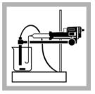
8. Using the Digital Titrator delivery knob, dispense the PAO Titrant Solution in 5 to 10 digit increments while noting the downward reading. If the chlorine content of the sample is high, add titrant at a faster rate.
