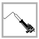
1. Install the Phenylarsine Oxide (PAO) Cartridge, 0.00564 N. Flush the Digital Titrator delivery tube by turning the delivery knob to eject a few drops of titrant. Reset the counter to zero and wipe the tip.
