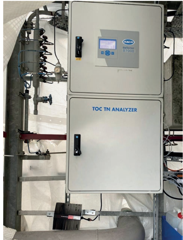
BioTector B7000 analyser for the determination of TOC, VOC and TN
