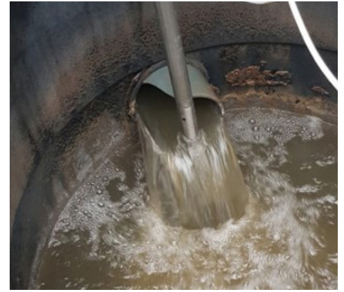
The Hach H 2 S sensor placed directly in the raw sewage in the inlet of the well.
