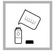
8. Prepare the blank: Rinse a sample cell and cap three times with sample. Fill the sample cell to the 10-mL mark with sample. Close the sample cell.
