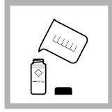
2. Prepare the sample: Rinse a sample cell and cap three times with sample. Fill the sample cell to the 10-mL mark with sample.
