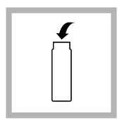
2. Add in quick succession to a dry reaction tube: 1.3 mL sample, 1.3 mL solution A, 1 tablet B.
