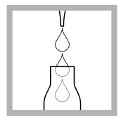
Carefully pipet 0.2 mL of solution D.
