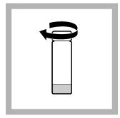
3. Close immediately the reaction tube. Do not invert.
