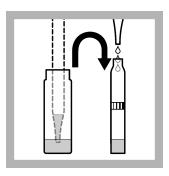
Carefully pipet into the Vial Test: 0.5 mL of digested sample.
