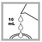
**21. Prepare the blank:** Fill a dry sample cell with 10 mL of chloroform. Put the stopper on the sample cell.
