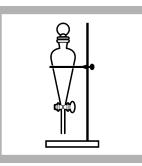
18. Put the funnel in the stand. Do not move the funnel until the timer expires.If there is cadmium in the sample, the bottom (chloroform) layer becomes orange or pink.
