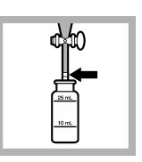
**19. Prepare the sample:** Put a cotton plug the size of a pea into the funnel delivery tube. Slowly drain the bottom (chloroform) layer into a dry 25-mL sample cell. Put the stopper on the sample cell. The Cd-dithizone complex is stable for more than 1 hour if the sample cell is closed tightly and kept out of direct sunlight.
