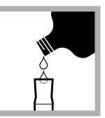
6. Prepare the DithiVer solution: Add 30 mL of chloroform to a 50-mL mixing cylinder.
