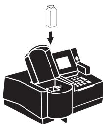
11. Place the prepared sample into the cell holder. Close the light shield. Results in mg/L manganese (or chosen units) will be displayed.
