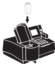
9. When the timer beeps, place the blank into the cell holder. Close the light shield.
