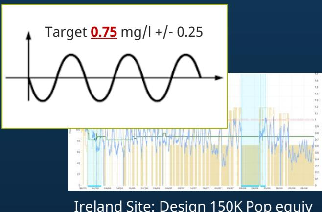
Customer had existing final eff phosphax and dosed into PST effluent. Simply added SC4500 to final effluent analyser to upgrade dose strategy
