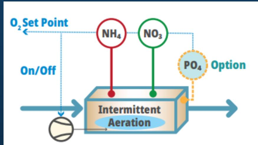
**RTC-NDN** : for controlling aeration on/off in intermittent operation.
