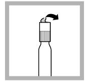
1. Sample cuvette: Carefully remove the foil from the screwed-on DosiCap Zip.
