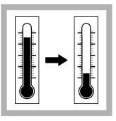
8. When the timer expires, set the reactor power to off. Let the temperature decrease for about 20 minutes to 120 °C (248 °F) or less.
