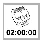
**7.** Keep the vial in the reactor for 2 hours.
