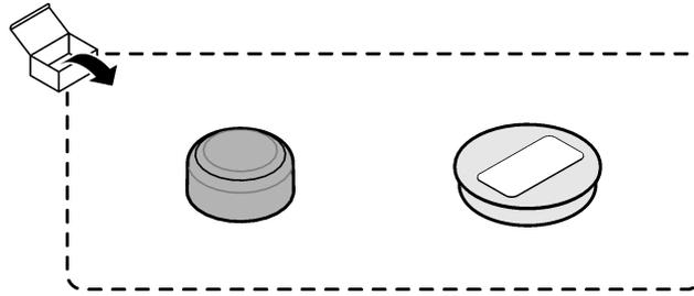
**EN:** Replace the sensor cap and iButton® at the same time. The iButton® updates the probe calibration for the new sensor cap.
