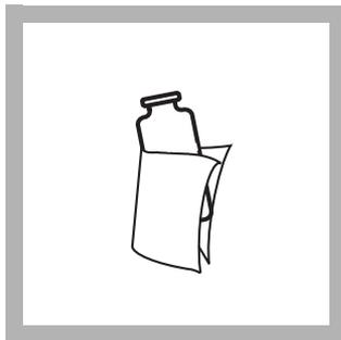
**9.** When the timer beeps, wipe the cells with a damp towel, followed by a dry one, to remove fingerprints and other marks.
