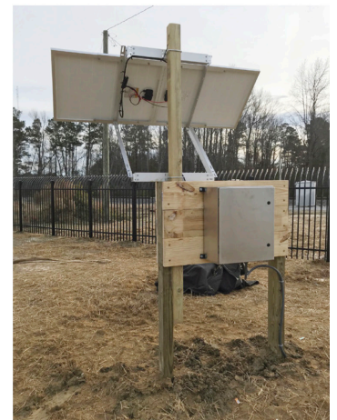
FL1500 with BL9000 bubbler installed in locations in North Carolina (US). Solar powered installation allows for use where no electrical power is available.
