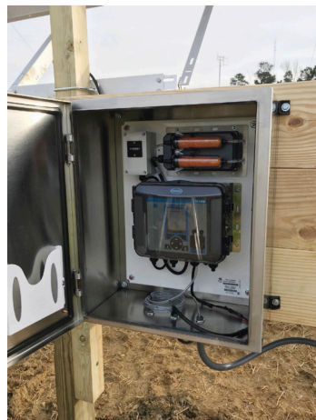
FL1500 with BL9000 bubbler installed in locations in North Carolina (US). Solar powered installation allows for use where no electrical power is available.
