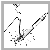
3. Rinse the probe with deionized water. Dry the probe with a lint-free cloth.
