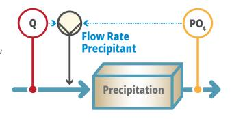
Precipitant has to be well mixed with the wastewater stream before
