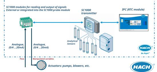
RTC modules are installed on an industrial PC. The site PLC receives analytical data from SC4500 Modbus, Ethernet IP, Profibus, Profinet or analogue (0/4...20mA). The IPC hosting the RTC modules communicates to SC4500 via Modbus TCP/IP (LXZ515.99.B0002)
