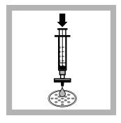
**9.** Filter slowly the incubated sample, discard the filtrate and wipe off any water drops adhering to the membrane filter.
