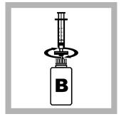
**14.** Screw the adapter **loosely** onto the bottle containing **solution B** and remove the cap. Screw the syringe with the membrane filter onto the bottle.
