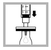
**17.** Filter the contents of the syringe carefully into the **sample** cuvette.
