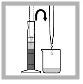
**4.** Use a transfer pipette to transfer the supernatant liquid into a glass beaker.
