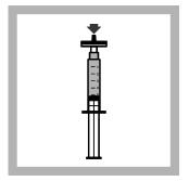
**8.** Screw on the membrane filter (LCW904).
