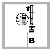
**11. Slowly** draw **solution B** through the membrane filter into the syringe until it reaches the **4.6 mL** mark.
