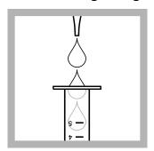
extension: **4.3 mL** activated sludge suspension and **0.5 mL** buffer **solution A**.
