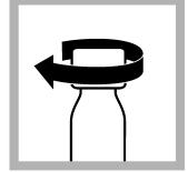
**4.** Close the cuvette and keep it in a **dark place** at room temperature (20–25° C (68–77° F)). Check the cuvette for a red coloration after 30, 45 and 60 minutes.
