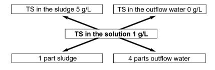
Pipet into the reaction tube: 2 mL sludge + 8 mL outflow water and mix
