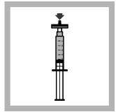
**12.** Screw on the membrane filter (LCW904).
