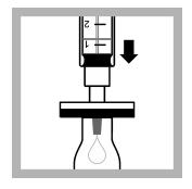
**13.** Filter the contents of the syringe **carefully** into the sample cuvette. Close the bottle containing solution B **securely** after use.
