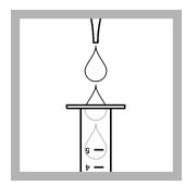
5. Pipet into the first syringe extension (Reference value):
