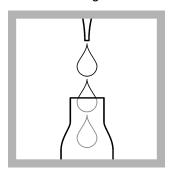
3. Use a transfer pipette to fill the cuvette to the brim with sample (make sure that no air bubbles remain in the cuvette).
