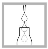
2. Pipet into the cuvette test: 0.6 mL of buffer solution A.
