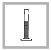
**2.** Fill a 25 mL measuring cylinder with activated sludge.
