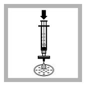
**13.** Filter the incubated sample, discard the filtrate and wipe off any water drops adhering to the membrane filter.
