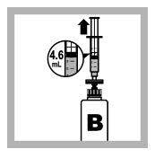
15. Slowly draw solution B through the membrane filter into the syringe until it reaches the 4.6 mL mark. Close the bottle containing solution B securely after use.
