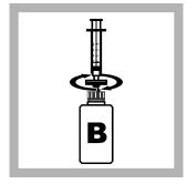
10. Screw the adapter loosely onto the bottle containing solution B and remove the cap.
