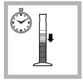
Allow the activated sludge to settle for 30 minutes.
