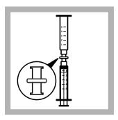
**1.** Set-up: Use the adapter to join syringe and syringe extension.
