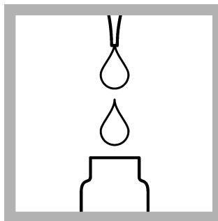
2. Use a pipet to add 0.2 mL of sample to the test vial. Immediately continue to the next step.
