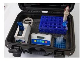
We recommend that every PhotonMaster Luminometer be stored and operated in its supplied carrying case, which also includes a space for the PhotonMaster Bluetooth Module and all the other equipment needed to carry out LuminUltra's test protocols. Contents normally include:
