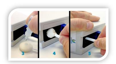
**DRYING**: Using a new dry swab, repeat the 6x clockwise / counter clockwise motion. Pull the swab and feel for dampness. If damp, use a new swab and repeat twisting steps. Continue to use new clean swabs until the swab comes out dry. This usually requires three swabs.
