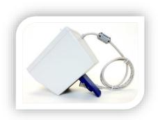
LuminUltra recommends that the PhotonMaster be cleaned at least on an annual basis. Please use only the approved Luminometer Cleaning Kit (LCK) or Luminometer Maintenance Kit (LMK) that is furnished by LuminUltra, which includes 5 foam swabs and cleaning fluid. Never use sharp or abrasive materials for cleaning the PhotonMaster chamber, as this can compromise the sensitive optics of the device!
