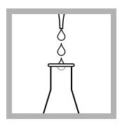
**7.** Add 5 drops of 5.25 N Sulfuric Acid Standard Solution.
