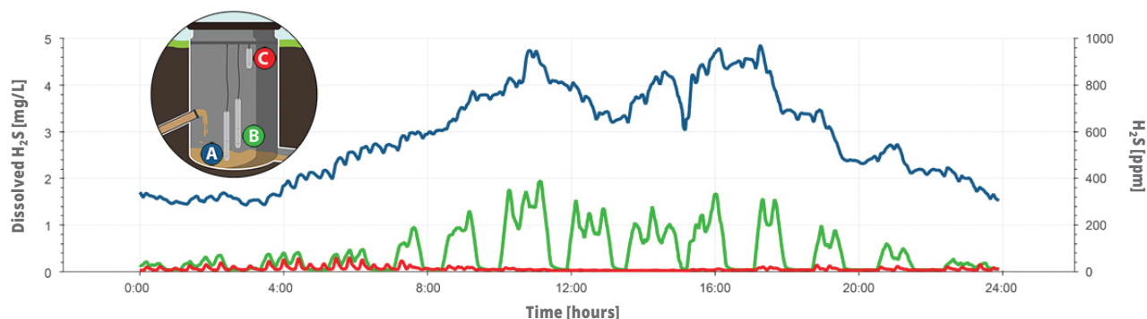
Figure 3. This chart shows differences in continuous readings from a liquid-phase sensor installed directly in the wastewater flow (blue) vs. gas-phase sensors installed just above the surface of the water (green) or near the top of a manhole (red). Notice the lower overall readings and periodic dropout of H 2 S values on the green line, representative of differences between pumping inactivity and turbulent flows that release more H 2 S gas. Note how measurements taken near the top of the manhole do not reflect the highest incidences of H 2 S.
