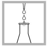
4. Add 2.0 mL of 5.25 N Sulfuric Acid Solution to the flask.
