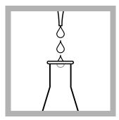
6. Let the sample cool to room temperature. Add 2.0 mL of 5.0 N Sodium Hydroxide Solution to the flask.
