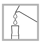
8. Pour the sample into a 25-mL graduated cylinder. Adjust the volume to 25 mL by rinsing the flask with deionized water and pouring the rinse water into the cylinder.
