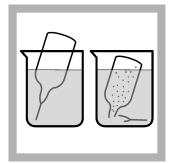
2. Prepare the blank: Pour at least 40 mL of deionized water in a 50-mL beaker. Fill one SPADNS Fluoride Reagent AccuVac Ampul with deionized water. Keep the tip immersed while the Ampul fills completely.
