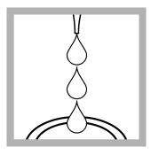
4. Use a pipet to add 2.0 mL of SPADNS Reagent Solution into each sample cell.
