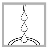
2. Prepare the blank: Use a pipet to add 10.0 mL of deionized water to a sample cell.
