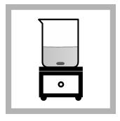
**9.** Add a stir bar and put the beaker on a magnetic stirrer. Stir at a moderate rate.
