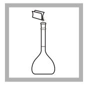
1. Prepare a 15% Sodium Acetate Solution: Add 150 g of Sodium Acetate to a 1000-mL volumetric flask.
