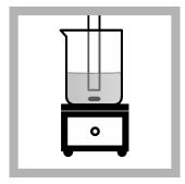
**10.** Put the probe in the solution. Do not let the probe touch the stir bar, bottom or sides of the container. Remove the air bubbles from under the probe tip.
