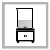
**8.** Add a stir bar and put the beaker on a magnetic stirrer. Stir at a moderate rate.
