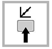
**12.** Push **Calibrate**. The standard solution value is shown.
