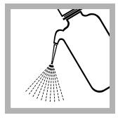
**9.** Rinse the probe with deionized water. Dry the probe with a lint-free cloth.
