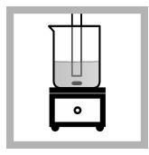
**11.** Put the probe in the solution. Do not let the probe touch the stir bar, bottom or sides of the container. Remove the air bubbles from under the probe tip.
