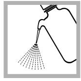
**10.** Rinse the probe with deionized water. Dry the probe with a lint-free cloth.
