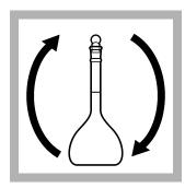
**3.** Put in the stopper. Invert the flask to mix well.
