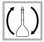
**3.** Put in the stopper. Invert the flask to mix well.
