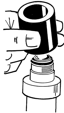
FIGURE 4-12 Placing Guide on Sensor
