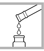
**10.** Pour 10 mL from the volumetric flask into a second sample cell.
