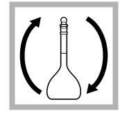
**4.** Put the stopper on the volumetric flask. Invert a minimum of seven times to mix.
