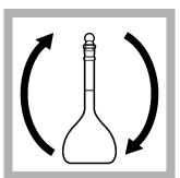
8. Put the stopper on the volumetric flask. Invert a minimum of seven times to mix.
