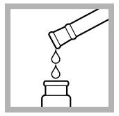
**5.** Pour 10 mL from the volumetric flask into a sample cell.
