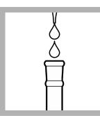
6. Prepare the sample: Use a pipet to add 1.0 mL of Chlorine Dioxide Reagent A into a second 25-mL volumetric flask.
