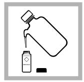
2. Prepare the blank: Fill a sample cell to the 10-mL mark with deionized water.
