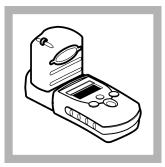
**18.** Install the instrument cap over the cell holder.
