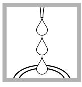
**6.** Add 12 drops of Alkaline Cyanide Reagent Solution to each sample cell.
