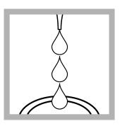
**8.** Add 12 drops of 0.1% PAN Indicator Solution to each sample cell.
