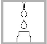
2. Prepare the blank: Add 0.1 mL of ammonia-free water to one AmVer™ Diluent Reagent Test 'N Tube for High Range Ammonia Nitrogen.
