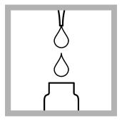
3. Prepare the sample: Add 0.1 mL of sample to one AmVer<sup>™</sup> Diluent Reagent Test 'N Tube for High Range Ammonia Nitrogen.
