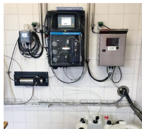
Fig. 2: EZ4004 online titrator from Hach
