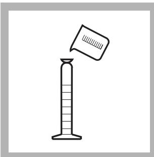
3. Fill a 25-mL graduated mixing cylinder to the 20-mL mark with sample.
