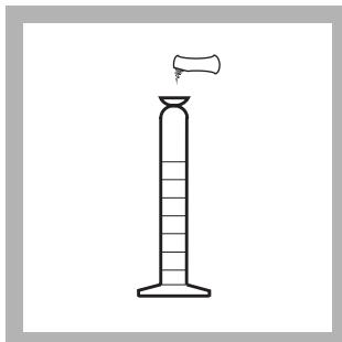
4. Add the contents of one ECR Reagent Powder Pillow for 20-mL sample size. Stopper. Invert several times to dissolve powder. Then press the soft key under **START TIMER**. A 30-second reaction period will begin.
