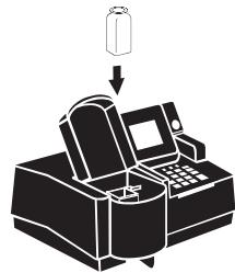
12. Immediately place the prepared sample into the cell holder. Close the light shield. Results in mg/L aluminum (or chosen units) will be displayed.
