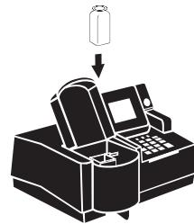
10. Within five minutes after the timer beeps, place the blank in the cell holder. Close the light shield.
