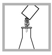
**6.** Add the contents of one Phenolphthalein Indicator Powder Pillow. The indicator is not necessary if a pH meter is used.
