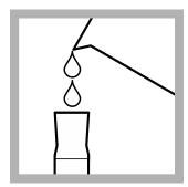
**3.** Use a graduated cylinder or pipet<sup>2</sup> to measure the sample volume from Table 1 on page 4.
