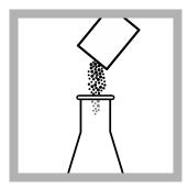
**6.** Add the contents of one Phenolphthalein Indicator Powder Pillow. The indicator is not necessary if a pH meter is used.
