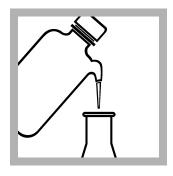
**5.** If the sample volume is less than 100 mL, dilute to approximately 100 mL with deionized water.
