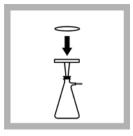
3. Set up the Membrane Filter Assembly. Use sterile forceps to place a membrane filter, grid side up, in the assembly.
