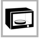
7. Label the petri dish with the sample number, dilution and date. Invert the petri dish and incubate at 35 ± 0.5 °C for 24 hours.
