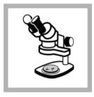
**8.** Remove the dish from the incubator. Count colonies on membrane filters using a 10–15X microscope.
