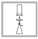
5. Turn off the vacuum and lift off the funnel top. Remove the membrane filter, using sterile forceps. Still using the forceps, transfer the filter immediately to the previously prepared petri dish.
