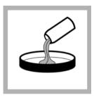
2. Invert ampules two or three times to mix broth. Open an ampule of m-TSB/USP or use an ampule breaker if necessary. Pour the contents evenly over the absorbent pad. Replace the petri dish lid.
