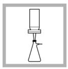
4. Invert the sample for 30 seconds, approximately 25 times, to make sure it is well-mixed. Filter the appropriate volume through the sterile 47 mm, 0.45μm, gridded membrane filter. Apply vacuum and filter the sample. Rinse the funnel walls three times with 20–30 mL of sterile buffered dilution water.
